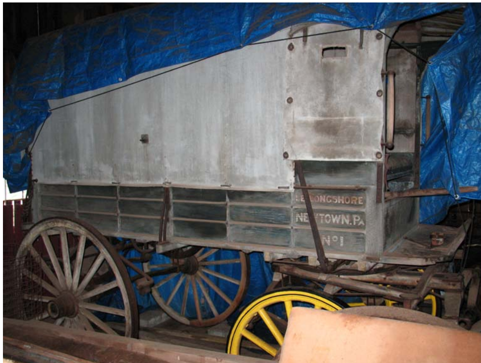
Photo of the market wagon owned by Ida Longshore of Newtown, PA. Ida Longshore had a farm on Washington Crossing Road, just North of Goodnoe's corner. This wagon was made by the Randall Carriage Factory in Newtown circa 1900. Ida used this wagon to haul produce to the farmer's market in Philadelphia. The wagon was pulled by two horses and it stands 9' high and is 12' long. The wagon is in the collection of the Newtown Historic Association.
